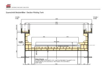
Above and beyond protection against thermal and mechanical stresses, brick linings offer improved chemical resistance since they prevent the direct contact of the medium to the impermeable membrane layer.
